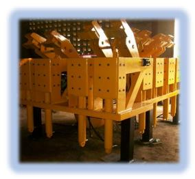
This **8-Mould Interlocking Brick Making Machine** as the name suggests has 8moulds thus capable of producing 8 bricks at a time. It is used to produce interlocking bricks for building construction.
