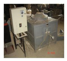
The **Salt Bath Furnace** is a furnace designed to carry out Austenitising and Austempering processes using a molten salt medium. It is used for the production of Austempered Ductile Iron.
