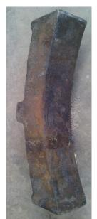
"As-Cast" Train Brake Shoe is an alloy of iron, carbon and silicon (grey cast iron). It is used as break shoes for locomotives.
