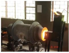
The **100kg Rotary Furnace** is used for melting cast iron. It is the most flexible and universal design of equipment to recycle cast iron and aluminum scraps. They are ideal for making heat resisting and other alloyed cast iron castings. Grey, nodular or malleable cast iron can be produced with high analytical accuracy at a low investment cost.
