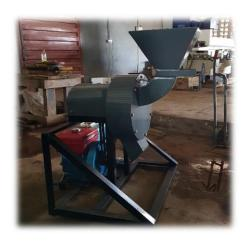
The **Hammer Mill** has a hopper through which raw laterite from site is fed into the milling chamber and through the mechanism of hammer milling, the laterite is grounded. This mill is useful for grinding raw laterite from the site.
