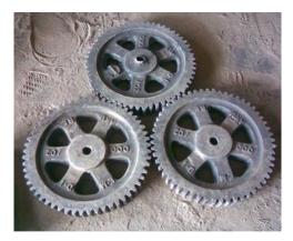
The **Bull Gear** is an alloy of iron, carbon and silicon (grey cast iron). They are used as gear components for heavy duty usage such as in Cranes and heavy- duty haulage. Load Bearing Capacity of 1Ton. (Ø 400 X 53 MM).
