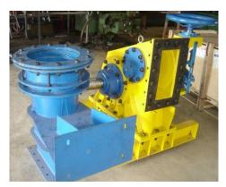
The **35KW Small Hydropower Turbine** is a crossflow impulse hydro power turbine developed through reverse engineering at EMDI Akure. It converts the energy in a flowing river at appropriate elevation into a rotational power which is later converted to electrical power through a generator. It is used to generate electricity.
