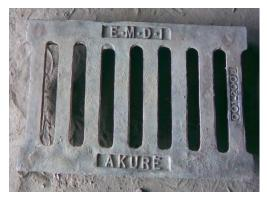
**Channel Grating** is an alloy of iron, carbon and silicon (grey cast iron). It is used to cover drainages giving access to vehicles. Carbon in the structure is flaky. Maximum load bearing capacity is 350KN
