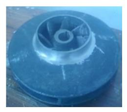
The **Water Pump Impeller** is an alloy of iron, carbon and silicon and manganese (grey cast iron). It is used as a major component of industrial water pump.
