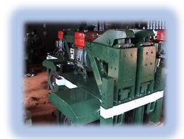
This **twin interlocking brick making machine** is used for producing bricks. The mould type determines the brick shape. They are used to produce interlocking bricks for building construction.
