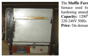
The **Muffle Furnace** is a non-melting, heat-treatment furnace used for heat treatment process such as hardening annealing, tempering, brazing, ageing etc. Capacity: 1200°C Maximum Temperature 1000° C
