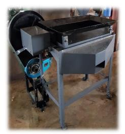
The **Sieving Machine** consists majorly of a wire mesh on which grounded laterite is further reduced into smaller particles by the sieving process. It is used to sieve laterite into finer particles.
