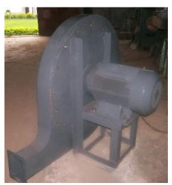
The **Industrial Blower** is a mechanical device for moving air or other gases and is a one of the major accessories of the Rotary furnace. This is used to generate air current for fuel combustion in the operation of Rotary furnaces. It can equally be used in any application that requires high flow of air current for its operation.
