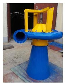
The **10kw Propeller Hydro Turbine** is a reaction-type hydropower turbine which operates at a relatively low head with high efficiency. It is used for power generation through the conversion of mechanical energy (of large volume of water) to electrical energy through the use of alternators. Head 5.5m. Flow Rate 220L/s.
